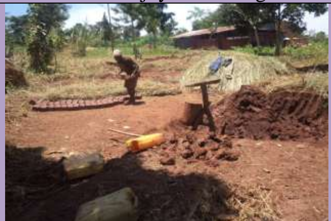
Ongoing work of school Brick making
